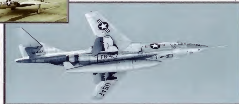
▶ Flaps down The Voodoo was built to fly very fast, but its large split flaps and leading-edge flaps gave it good handling at low airspeed, even when fitted with large external fuel tanks.
